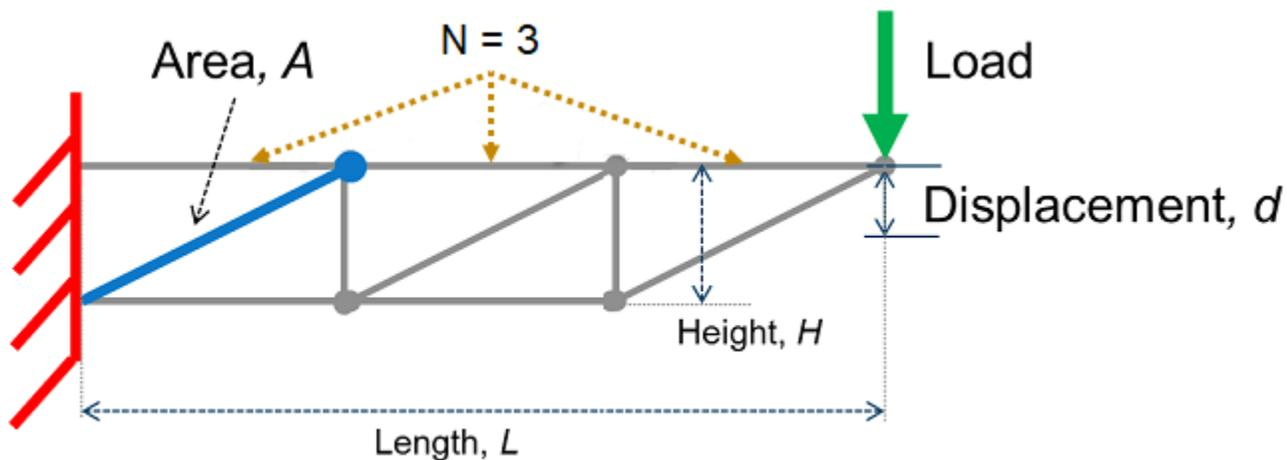
The truss bars are made of a linear elastic material with uniform density. The cross-section area  $A$  of the bar highlighted in blue (see figure) can vary. All other parameters, including the uniform cross-section areas of the other bars, are fixed. Obtain the displacement of the tip by using small and linear displacement assumptions.
