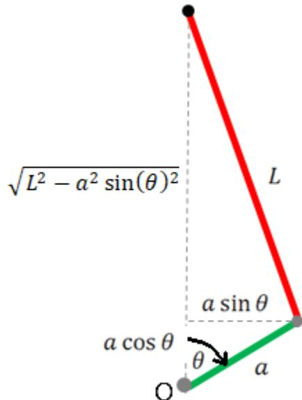
The height of the piston relative to the origin is  $H = a \cos \theta + \sqrt{L^2 - a^2 \sin(\theta)^2}$ . Define the piston height as a symbolic function by using the syms function.
