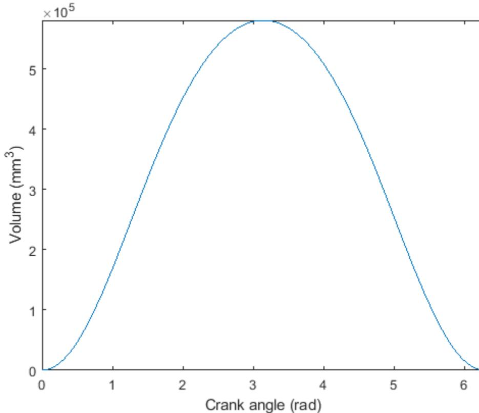
The piston volume is smallest when the piston is at TDC and the crank angle is  $0$  or  $2\pi$ . The piston volume is largest when the piston is at BDC and the crank angle is  $\pi$ .
