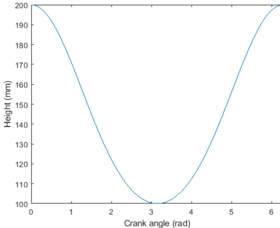
The piston head is highest when the piston is at TDC and the crank angle is  $0$  or  $2\pi$ . The piston head is lowest when the piston is at BDC and the crank angle is  $\pi$ .
